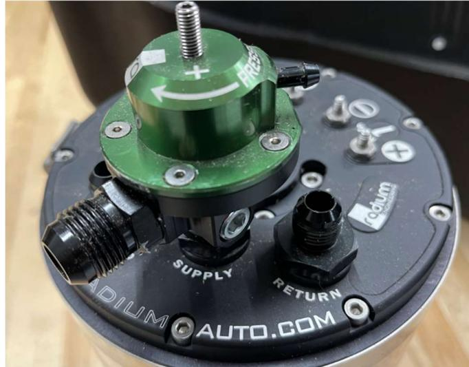
This is an example of a DMR attached to the supply port of the MPFST.
