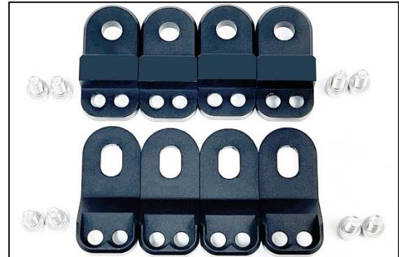
5. For the 2021+ Ford F150 V8 (only), install these specific mounting feet in the orientation shown. Apply a medium-strength thread locker to the 8 screws and secure using a 4mm Allen wrench.
