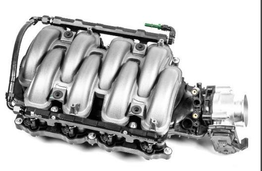
15. Because of the IMRC assembly on this application, the crossover hose routes along the frontside of the intake manifold.
