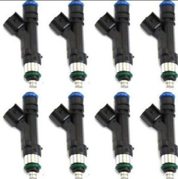
12. Prior to reinstalling the 8 OEM fuel injector retaining clips, it is important to position the fuel injectors exactly how they came from the factory. This is important for the injector wiring length to properly reach, but also for performance. For instance, the fuel injector from the 2021+ Ford F150 (shown) has a specific spray pattern that will not atomize as effectively if not clocked accordingly.
