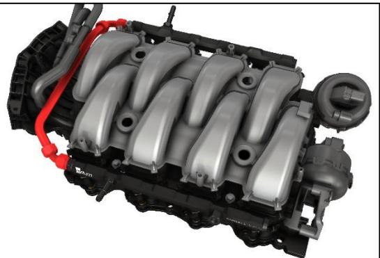
16. For the truck intake manifolds, the crossover hose can be routed along the backside, as shown.
