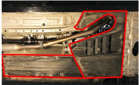
3. Find the mounting bracket and three M8X1.25mm button head screws in the kit. Using a 5mm Allen hex wrench, secure the bracket to LH tunnel over the hard lines near the transmission.
