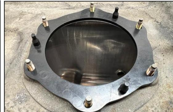
35. When installing, tilt the assembly so the fuel level float enters the tank first. For all EVOS (1-6), the float will enter towards the center of the fuel tank. If this is accidentally installed 180 degrees out, the float will not have enough room inside the fuel tank to move.
