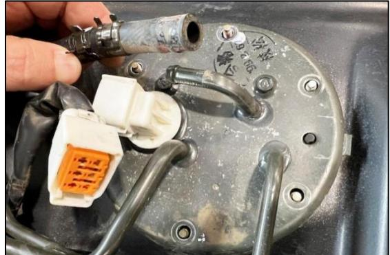
8. When removing the fuel pump from the tank, it will be necessary to tilt the assembly to get the fuel level sensor float out. Be careful not to damage the fuel level float arm. Pull the fuel pump out and set into a fuel safe bucket. Evolution 6 tank shown.
