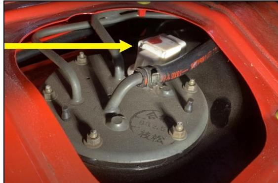
5. For the EVO 4-5-6, the fuel tank must be removed. Evolution 5 tank shown. NOTE: Once the Radium fuel hanger is installed, the tank will no longer need to be removed for servicing.
