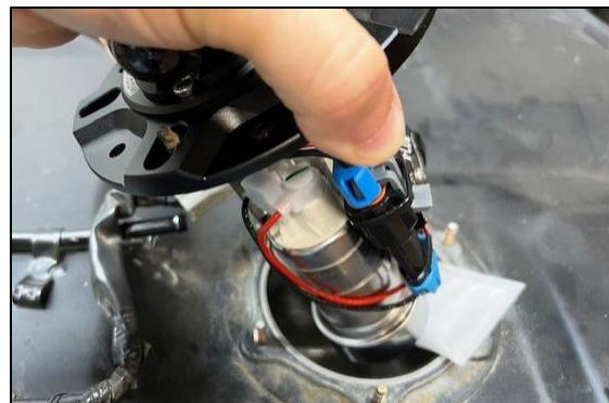
36. When lowering, be sure all internal components do not get hung up. Be sure to fully pull the 3 alignment rubber tabs out of the holes from the top side.
