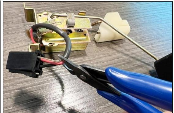
29. Slide the black rigid sleeve (shown) off the wires. The OEM connector and the wiring sleeve will NOT be reused.
