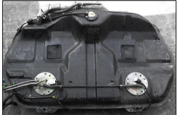
6. It is recommended to clean the top of the fuel tank and the surrounding area. This will prevent loose dirt from falling into the gas tank.
