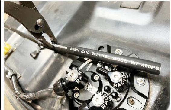
47. Lineup the 5/16" EFI hose to the "CROSSOVER" barb fitting. Make a cut line on the hose. Cut the 5/16" EFI hose at the mark.
