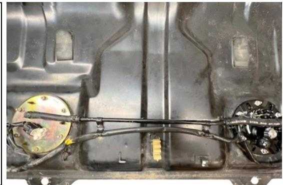
44. Install the ring terminals to the appropriate studs.
