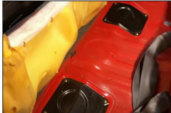
4. To depressurize the system, unplug the fuel pump connector. NOTE: The fuel pump on the EVO 1-5 is located on the RH side of the fuel tank. The fuel pump on the EVO 6 is located on the LH side of the fuel tank.
