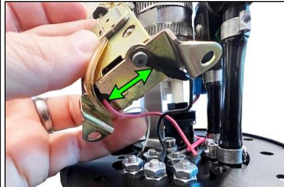
32. When mounting the 2-bolt sensor, do not (mistakenly) have it flipped around 180 degrees.
