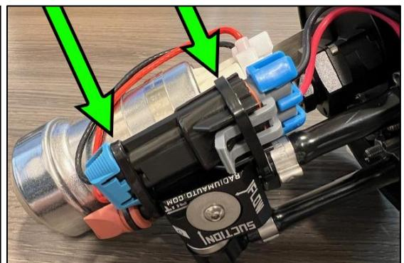
28. Pry the OEM metal stay up slightly to free the OEM wiring loom.
