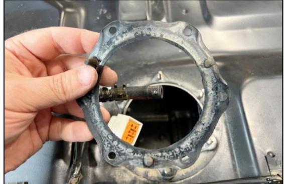
10. To unplug the black fuel level sensor connector, squeeze the tab and simultaneously pull.
