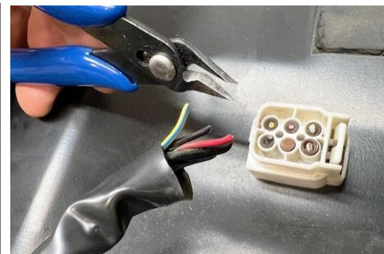
41. Strip the insulation off all 5 wires. As shown, be sure the thick gauge wires use the large heat shrink and the thin gauge wires use the small heat shrink. Extra parts may be present in the kit and can be used as spares.
