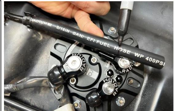
48. Secure the 5/16" crossover EFI hose using the other spring clamp. EVO 6 fuel tank shown.
