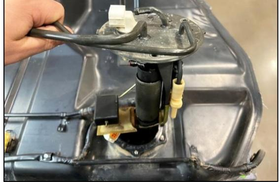
9. Carefully pry off the OEM gasket from the fuel hat. Although the original gasket could likely be reused, it is recommended to replace it as they typically become rigid and difficult to reinstall.
