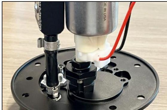
22. When securing the fuel pump, there is some adjustability put into the mounting bracket.
