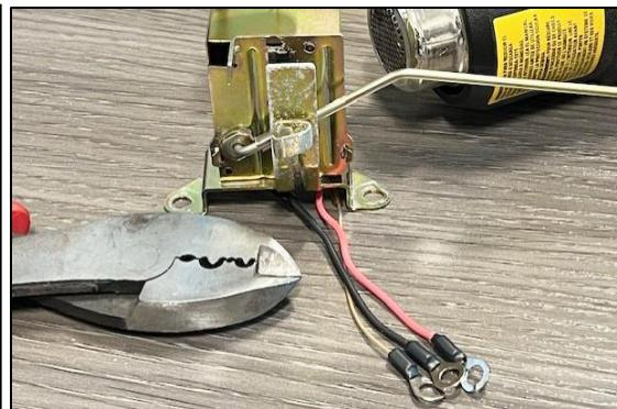
31. Using a small screwdriver, loosen the black ground ring terminal underneath the OEM fuel level sensor. Rotate all the way to the side (as shown) and tighten.
