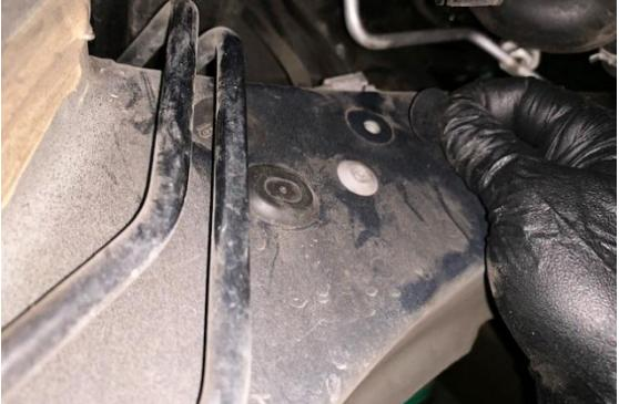
7. Using 14mm and 10mm wrenches, secure the fuel filter bracket to the chassis, as shown.
