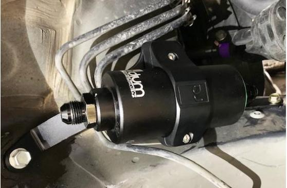
8. This picture is shown with hoses (not included) connected to the fuel filter.
