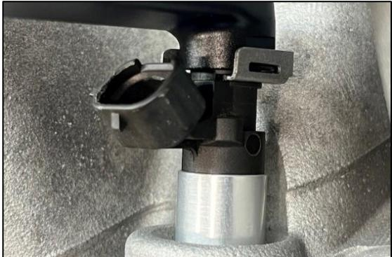
**18. Position and line up each fuel rail over the intake manifold. Press firmly down and verify that the lower injector O-ring seal is fully inserted and seated. Once everything is positioned correctly, reuse the 4 OEM screws (shown red) and tighten using a 10mm socket.**
