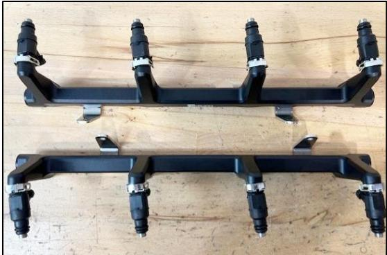
**17. There are machining features on each fuel rail injector port. These are designed specifically for the smaller retaining clips commonly used with popular Bosch Motorsport EV14 style injectors (shown).**
