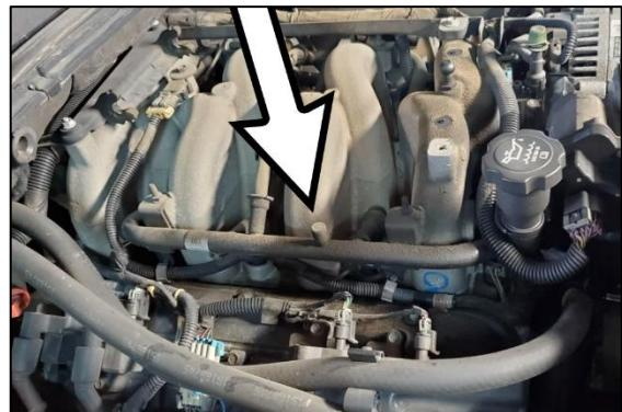
3. Disconnect the 8 injector connectors. Using a 10mm socket wrench, remove the 4 fuel rail screws. To prevent fuel from draining, keep all injectors installed to the fuel rails and carefully remove the entire assembly with the sub harness from the vehicle. Clean out any dirt or debris found in the intake manifold injector seat bores.
