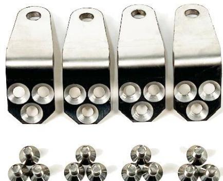
5. Install the 4 mounts in the orientation shown. Apply a medium-strength thread locker to the 12 screws and secure using a 3mm Allen wrench.
