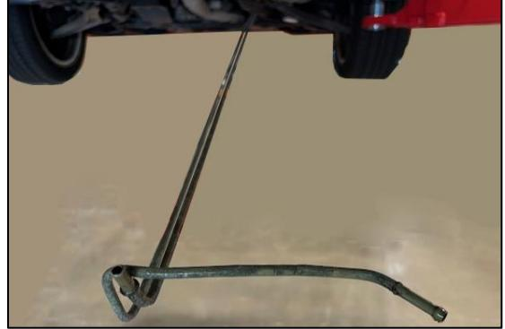
8. From the engine bay near the fuel filter location, separate the EVAP and return line by removing the clamp shown.
