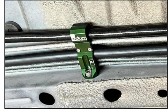
19. As shown, the next retainer is unique. It will still be secured to the chassis using an M6x1mm socket head screw and a 5mm Allen wrench. Tighten the small M3x0.5mm screws using a 2.5mm Allen wrench.
