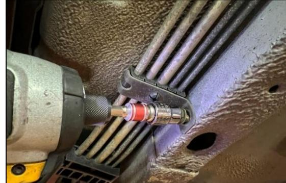
5. There is a fuel/brake line retainer that looks as shown. Remove it from the chassis using a 10mm socket. Pop the steel brackets from the plastic retainers. Pry the fuel/brake lines from the plastic retainers.
