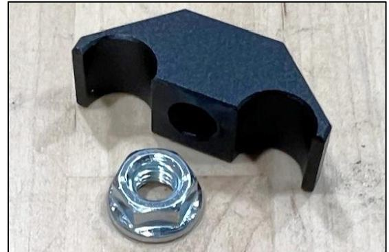
13. Using a 10mm socket, install the provided billet clamp and flanged nut to the firewall stud on the LH side of the EVAP fuel line (near the fuel filter).
