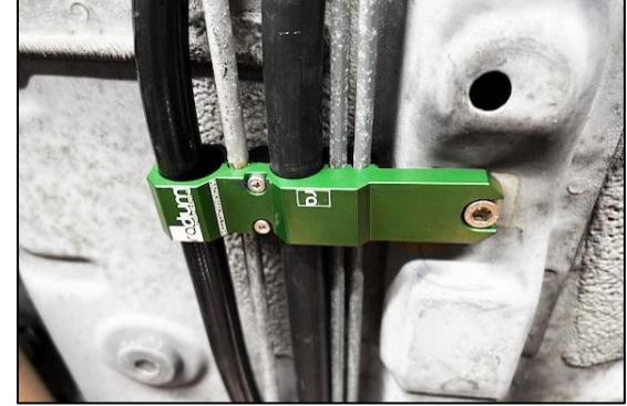
20. As shown, the next retainer is positioned around the corner, perpendicular to the others. It will NOT be secured to the chassis.
