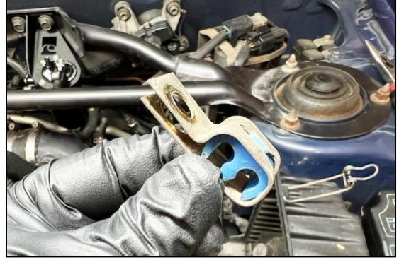
9. There are a couple of plastic retainers that secure the OEM fuel feed line, return line, and the EVAP line to the firewall. They are slightly difficult to reach. A pry bar will be handy.
