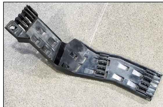
4. There are a couple of fuel/brake line retainers that look as shown. Remove them from the chassis using a 10mm socket. Pop the steel brackets from the plastic retainers. Pry the fuel/brake lines from the plastic retainers.
