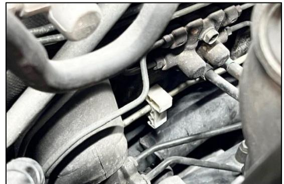
15. As shown, the front retainer will NOT be secured to the chassis. Tighten the small M3x0.5mm screws using a 2.5mm Allen wrench.
