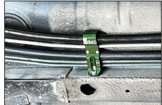
17. As shown, the next retainer will NOT be secured to the chassis. Tighten the small M3x0.5mm screws using a 2.5mm Allen wrench.
