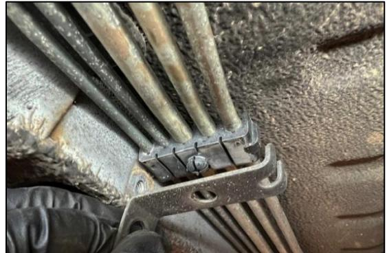
7. Allow the fuel/brake lines to hang temporarily.
