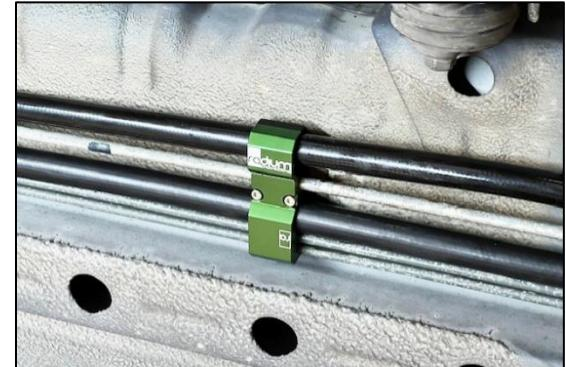
18. As shown, the next retainer will be secured to the chassis using an M6x1mm socket head screw and a 5mm Allen wrench. Tighten the small M3x0.5mm screws using a 2.5mm Allen wrench.
