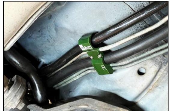
16. As shown, the next retainer will be secured to the chassis using an M6x1mm socket head screw and a 5mm Allen wrench. Tighten the small M3x0.5mm screws using a 2.5mm Allen wrench.
