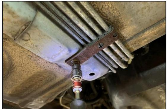
6. There are a couple fuel/brake line retainers that do not secure to the chassis. As shown, pop the steel portion from the plastic retainers. Pry the fuel/brake lines from the plastic retainers.
