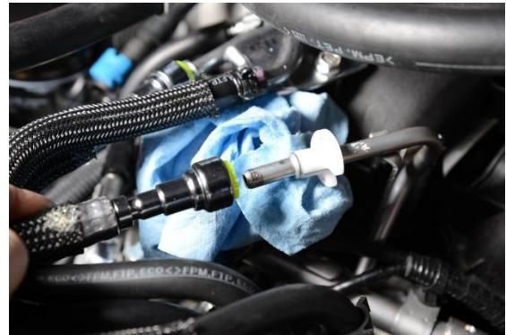
34. Some vehicles will use a barbed feed line on the HPFP pump, as shown.
