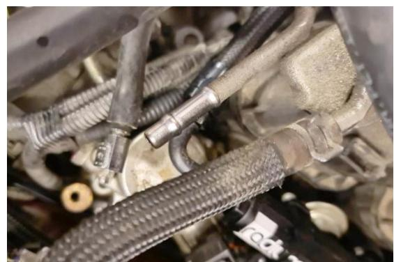
35. The two -6AN fuel lines from the Radium FPR are identical and cannot be crisscrossed. They can be connected to either the HPFP line or the port injection fuel line.
