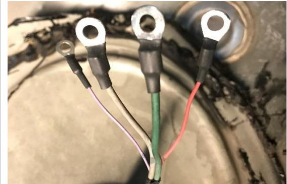
**22. Optional high-current wiring:** For high flow, high pressure fuel pumps, consider using Radium DIY wiring kit P/N: 17-0031 (shown) for each pump. This includes a dedicated fuse, relay, 10AWG wire, etc. It is recommended to use the OEM fuel pump wiring to trigger this fused relay power source for each pump.
