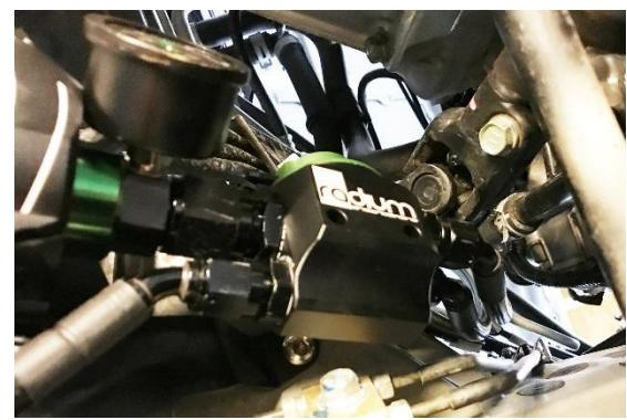
30. Secure the fuel filter heat exchanger section of the assembly to the mounting bracket using the four included M6 socket head bolts. Tighten using a 5mm Allen hex wrench.
