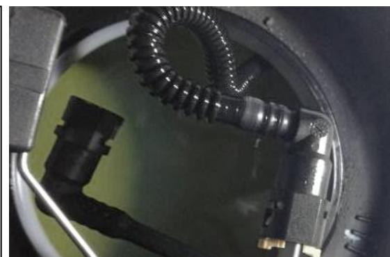
20. When installing, lean the assembly side to side to prevent the crossover hose and fuel level float from contacting the opening of the fuel tank.
