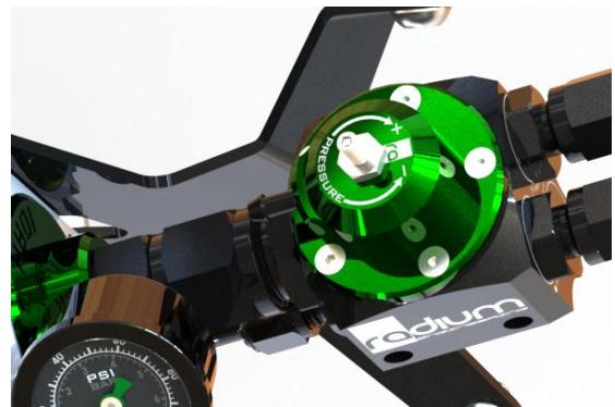
39(b). For newer kits (20-0966-0X) no tools are required to set fuel pressure. Simply turn the pressure adjustment knob until desired fuel pressure is achieved. The fuel pump(s) must be running to adjust pressure.
