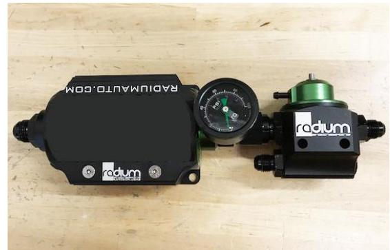
29. Find the 2 short (identical) 6AN PTFE hoses in the kit that have a 45-degree hose end on one side and a 90-degree hose end on the other side. Install the 45-degree hose end sides to the high pressure FPR ports.
