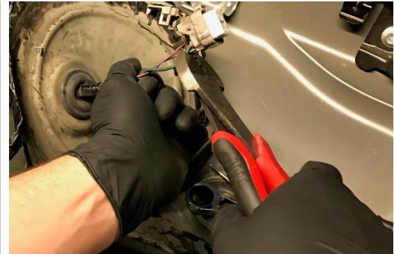
24. Cut two  $\frac{1}{4}$ " pieces of the small diameter shrink tube. Insert onto each sensor wire (two small gauge wires). Next, crimp on a small gauge (AWG) ring terminal to each wire. Slide the shrink tube over the crimped section of the ring terminal and shrink into place with a heat gun. Extra parts may be present in the kit and can be used as spares.
