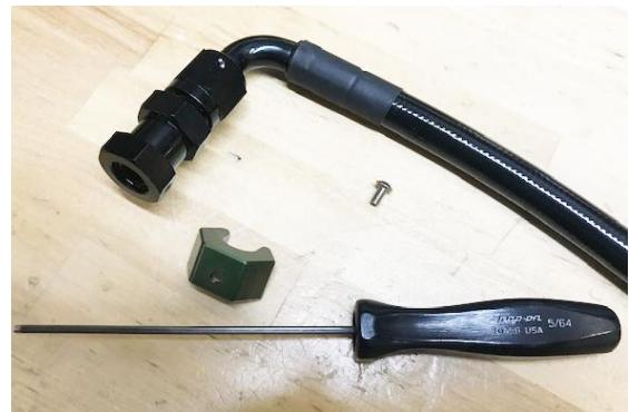
36. The procedure for connecting to aftermarket fuel rails will vary. For Radium Engineering 20-0111 fuel rails, one hose can be connected directly to the front port of the LH Radium Engineering fuel rail, as shown. NOTE: The rest of the parts from the fuel rail plumbing kit (including the crossover hose) will be reused.
