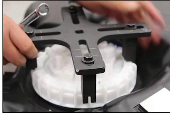
4. Before removing the OEM fuel pump housing, place an empty bucket nearby. There will be residual fuel in the gas tank and in the OEM fuel pump bucket. Slowly lift the canister straight up then tilt the fuel pump housing towards the right side to clear the level sender, as shown.
