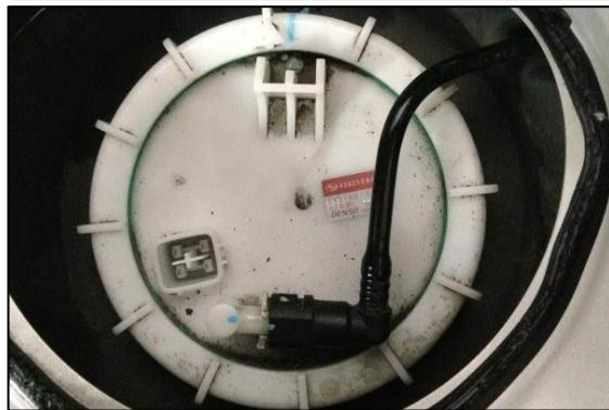
3. To allow extra room, the nearby rubber grommet can be removed and the OEM wiring harness can be pulled out for easier modification access later.
