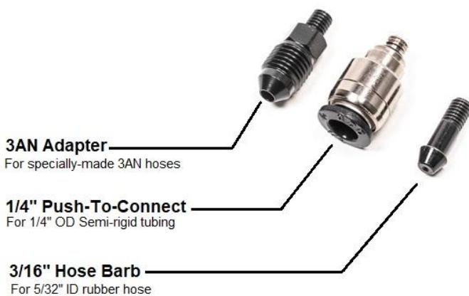
When installing the vacuum fitting, use a wicking thread locking compound, such as LOCTITE 290. If not available, any other medium strength thread locking compound can be used. Take care not to allow the thread locking compound in the air passage of the vacuum adapter. Simply finger tighten the fitting.
