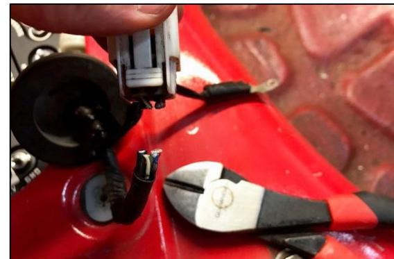
57. Cut the OEM external ground terminal off using diagonal cutters, as shown.
