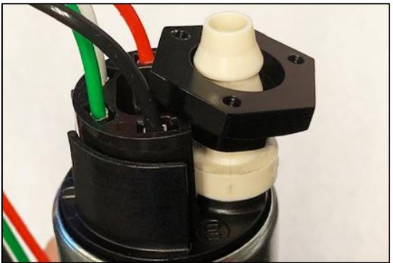
18. Next, slip the stainless steel retainers under the hose barb ridge closest to the end of the pump outlet opening. Be patient as this will take a little bit of work.
