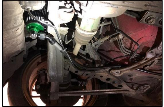
9. Use a 10mm socket and remove the factory fuel line covers and set aside.
