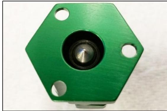
23. Apply a high-strength thread locking compound to the threads on the 3 included bolts. Line up the green fitting holes to the black fitting threads. Use a 2.5mm Allen wrench.
