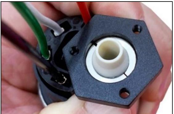
19. Place the included O-ring on the fuel pump outlet. Apply a petroleum-based lubricant to the O-ring.
