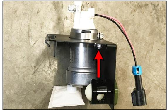
38. Find the OEM fuel level sender float/temperature sensor probe assembly.
