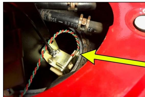
55. Check to be sure none of the electrical wires are getting pinched. Also check that the 8 OEM gasket holes line up with the corresponding threads.
