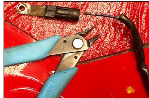
58. Unravel the electrical tape and remove the access cover rubber grommet from the wiring harness, as shown.
