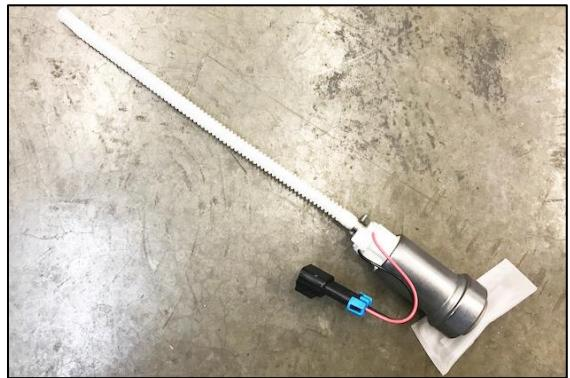
37. Insert the pump through the bottom side of the included lift pump baffle. NOTE: depending on the pump, it may save time to place one of the included worm drive clamps on the bottom side prior to inserting the pump.
