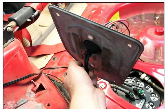
62. Use the large diameter shrink tube and large gauge (AWG) ring terminals to connect all fuel pump wires.
