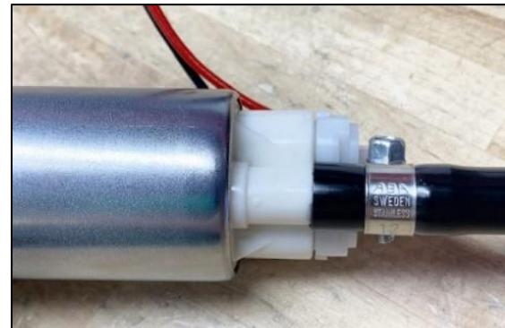
14. Determine how many fuel pumps will be installed. For single or dual fuel pump applications, block-off the unused ports on the underside of the triple pump block using the included 6AN ORB plug fittings and an 1/4" Allen wrench.
