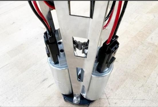
34. Before fully seating the FST canister to the top plate, correctly position the electrical wires. The black sensor ground wire should NOT enter the FST canister. The black connector with the green and white wires will be used for the fuel level/low fuel sensor.
