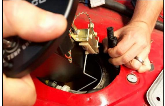
54. Find another person to help with this step as it is difficult. The fuel level sender will need to be pressed inward with an object to get it past the gas tank opening.
