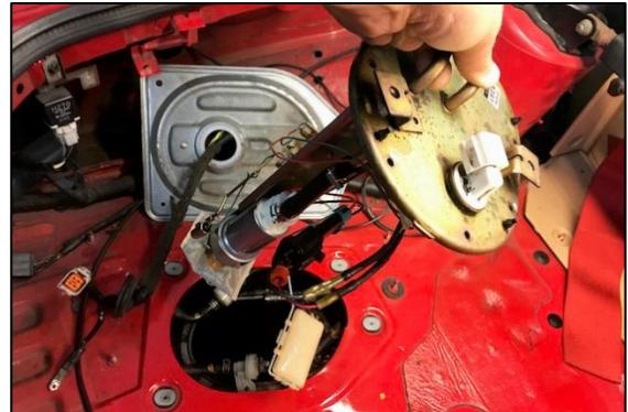
6. NOTE: If installing into a late model Mazda RX7 (FD), there will be a silver baffle on top of the internal sub tank, as shown. This metal plate must be removed. Both early and late model RX7s will benefit from the Radium Engineering baffle replacement in later steps.
