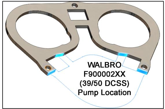
28. Install the brushless pump adapter bracket (pink) to the main pump bracket (yellow).
