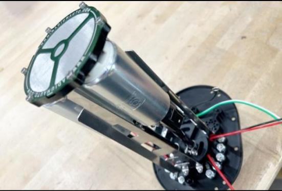
33. If using brushed pumps, plug in the fuel pump connectors.
