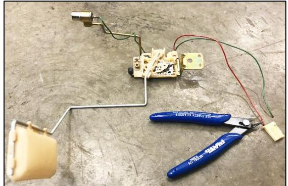
39. For flexibility, it is recommended to twist the 2 wires together.
