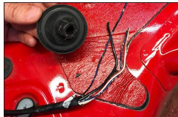
59. The OEM fuel pump power wiring will be reused for the lift pump. The OEM wiring does NOT need to be upgraded since the lift pump operates at very low pressure thus low current.
