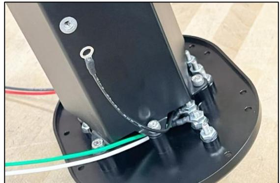
9. Using a 4mm Allen wrench, remove the 4 bolts that attach the FST canister to the top hat. Separate the two parts, as shown.
