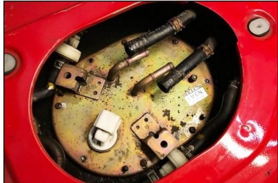
4. It is necessary to drain the tank to reduce fuel spills for an easier and safer installation.
