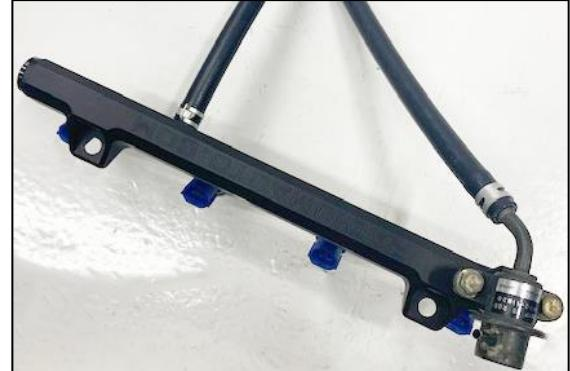
10. Lubricate the fuel injector top and bottom O-rings with oil. Fully insert the injectors into the Radium fuel rail bores.
