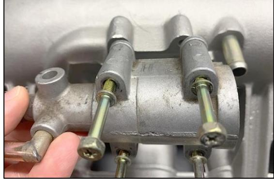
4. Using a 12mm socket wrench, remove the 2 fuel rail mounting bolts. Carefully pull the fuel rail from the engine.
