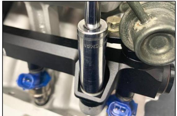
11. As a test, push the fuel injectors downward until they bottom out. Now inspect the injector upper O-rings and confirm they are still inserted into the fuel rail injector bores. Do NOT pressurize the fuel system until the proper height is achieved.
