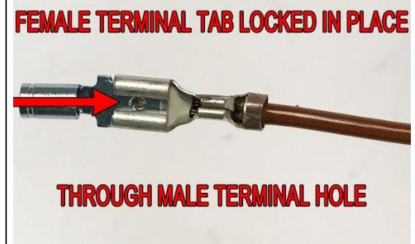
15. If using a Walbro F90000262 Fuel Pump, no adapter wiring harness is required as it uses the same terminals (shown) found on the BMW fuel pump.
