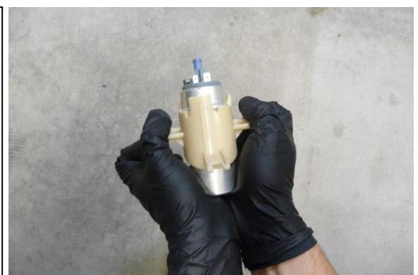
11. The following steps outline the use of spade terminals to connect to the 2 factory fuel pump wires. When performed properly, this connection method works very well.
