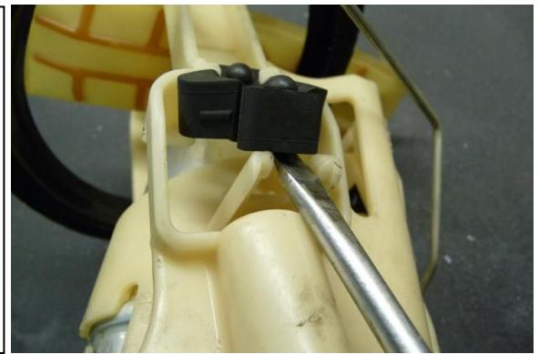
10. Take note of the clocking orientation of the plastic holder in respect to the fuel pump's outlet barb. To release the BMW fuel pump, pull the plastic tabs downward (as shown). The holder will come out the bottom of the pump.
