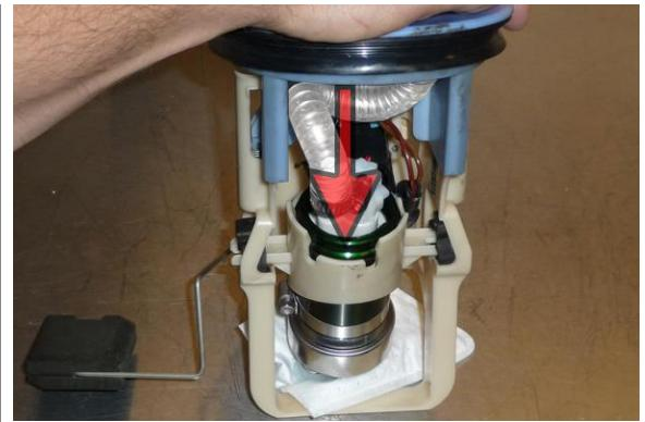
24. Be sure the gasket is installed before reinstalling into the tank.
