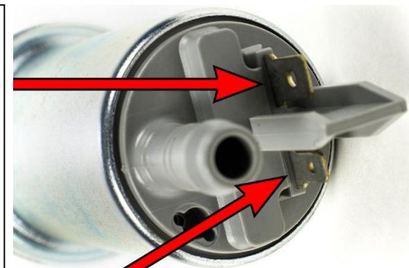
16. Crimp the male spade connectors as shown. Use the small 3/16" male spade on the black "-" wire and the larger 1/4" male spade on the red "+" wire. Gently give the wires a tug to confirm the crimp.
