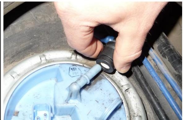
6. To unfasten the ring connection, BMW sells a special tool, P/N: 16 1 020. If not available, a rubber mallet hammer and punch will suffice. When spinning the ring counterclockwise a dab of glue will break free. If the ring is stubborn, get a second person to hit the opposing side of the ring simultaneously.
