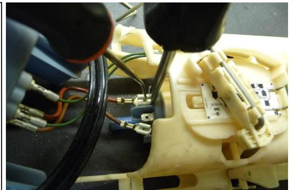
9. Carefully pry the rubber isolation grommets off each side of the fuel pump using your fingers and a screwdriver, as shown. These will be reinstalled later.
