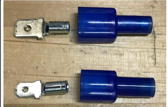
13. The OEM fuel pump wires use female spade terminals. Each of these terminals have tabs that lock into the holes of the male connectors. Depending on the force applied to the tabs when the terminals were removed, it is possible for them to be over bent. In this case, use a small pick to press the tab downwards (as shown in top picture).
