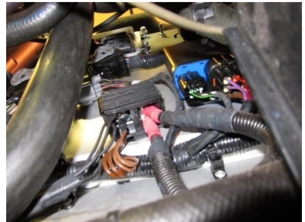
10. From the LH rear wheel well, locate the inertia safety switch in the engine compartment.
