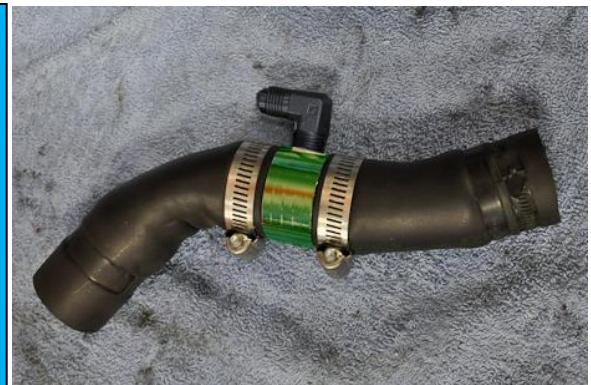
4. Rotate the fitting so that it is inline with the aluminum adapter pointing toward the inlet of the filler hose. Reinstall the fuel filler hose assembly into the vehicle.
