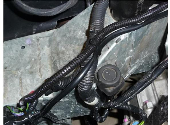
11a. For newer kits manufactured after August 2023, locate the single Weather Pak connector from the FST harness. Cut off the connector and strip the wire to expose the copper. The switched fuel pump wire terminal 3 on the inertia switch connector. Locate the Posi-tap connector in the kit and unscrew both ends. Put the slotted end around the terminal 3 wire. Push the trigger wire into the Posi-Tap connector. Tighten both ends together, as shown.
