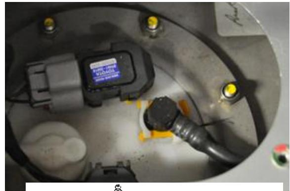
17. The final FST hose is the longest and has 90 degree hose ends.
