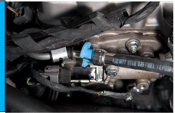
11. From the engine bay, install one of the SAE quick disconnect adapter fittings (shown) onto the shorter hose.
