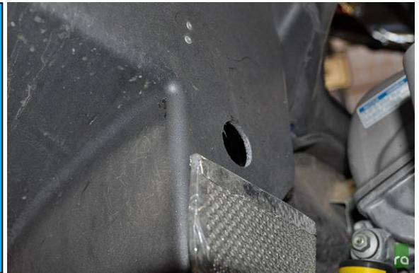
14. Locate the shortest hose in the kit and the remaining rubber grommet. Slide the grommet around the 90 degree hose end and push the straight hose end through the drilled hole from the trunk side.
