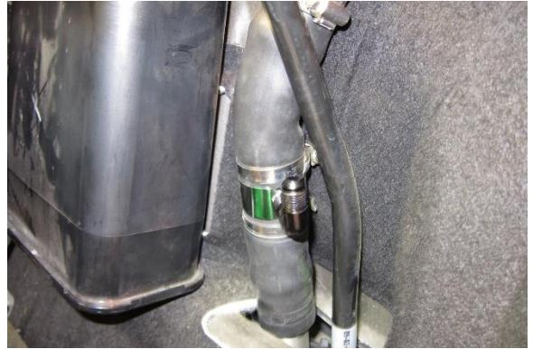
7. From inside the RH rear wheel well, locate the three fasteners on the frame rail holding the A/C line bracket in place. If the vehicle is not equipped with A/C, there will be 3 threaded holes in this location. NOTE: The Lotus 211 typically does not have these aforementioned threaded holes. Drilling and pulling three M6x1mm rivet nuts is required.
