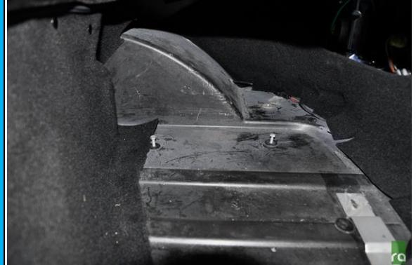
16. Eye up the bracket and scribe the inner wall through the hole on the upper left portion of the bracket and remove it from the trunk. Drill a  $\frac{1}{4}$ " hole through the wall into the rear right fender well. Note: Pending the accuracy of the hole drilled, it may need to be enlarged to be concentric with the FST bracket's mounting hole.
