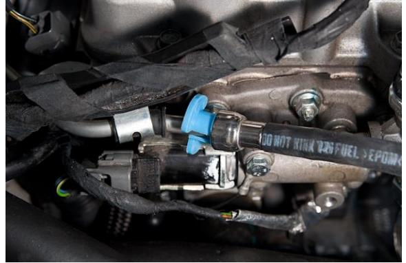
5. Find the rubber fuel filler hose on the lower RH side of the firewall from the engine bay. Loosen both OEM clamps and remove the hose from the vehicle, as shown.
