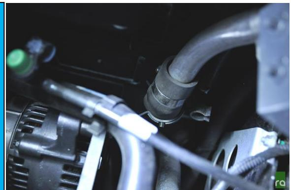
3. Cut a 1" section from the middle of the straight section of the filler hose, roughly 4.5 inches from the end that attaches to the fuel tank. This measurement may vary depending on Lotus model. Please double check before cutting.
