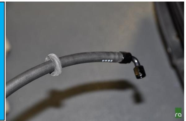
10. Using the included 5/16" SAE disconnect tool, remove the OEM fuel line from the fuel rail pipe. Insert the tool into the end of hose and apply pressure while simultaneously tugging on hose. The tool will release the SAE quick connect locking mechanism and the hose should slide off.
