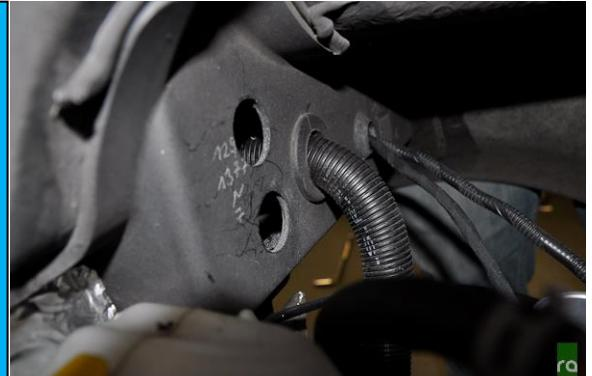
9. Locate the 2 longest preassembled hoses and two of the rubber grommets included in the kit. Slide the grommets over each hose as shown.
