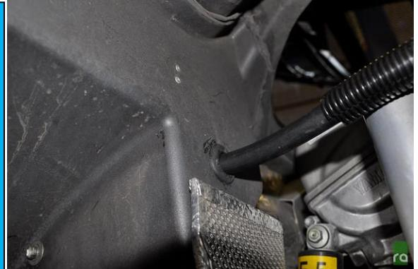
15. Locate the two M6x1.0mm floor mounted bolts on the right side of the trunk. Using a 10mm socket, remove these bolts and washers.
