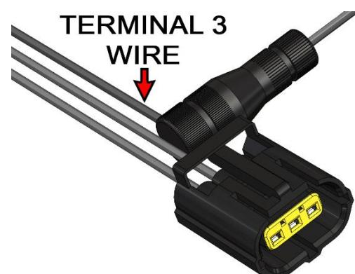
11b. For older FST install kits manufactured prior to August 2023, locate the jumper harness (shown) included in the installation kit.
