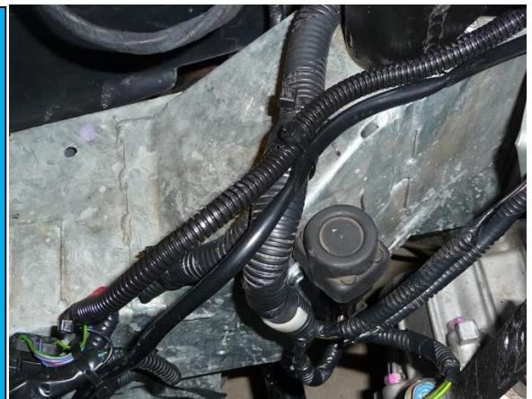
6. Unplug the connector from the inertia switch by squeezing the latch and pulling downward.
