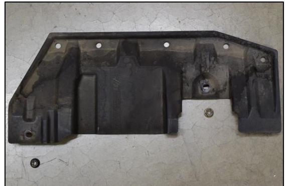
36. The center metal under tray brace (pictured) under the exhaust downpipe elbow and driveshaft needs to be removed temporarily. Remove the 4 bolts and drop the brace down.
