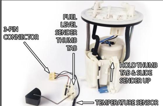
6. To install fuel pumps, the fuel hanger must be partially disassembled.
