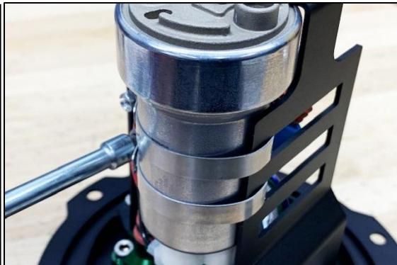
17. For dual 2-wire brushed pumps, install the extra harness ring terminals underneath the fuel hat to the “2-WIRE BRUSHED PUMP 2” studs labeled “12V+” (red wire) and “GROUND” (black wire). Tighten the lock nuts with a  $\frac{3}{8}$ " wrench. Plug in each fuel pump connector.
