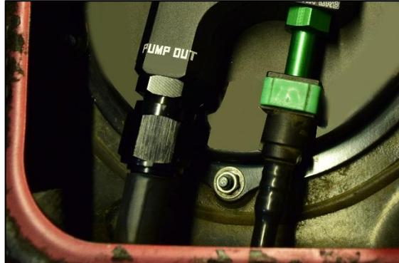
45. Torque the 5/16" SAE Male Fitting into either end of the PTFE hose included in the kit. If installing to a Radium fuel rail with a DMR installed onto the top port, make sure the 6AN male return fitting is pointing towards the left side of the vehicle. Loosely install the opposing hose end to the DMR's 6AN male fitting. NOTE: Hose routing will differ if installing onto a different brand pressure regulator.
