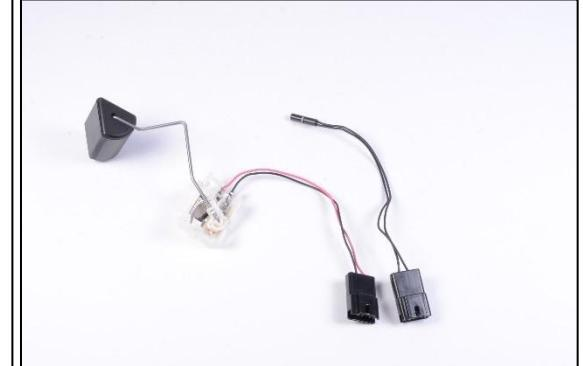
22. Place the fuel temperature sensor (shown red) on the fuel sensor mount (shown yellow). Slide the 2 included zip ties (shown green) in and out of the 4 slotted holes. Secure the OEM fuel temperature sensor and cut the zip tie tails.
