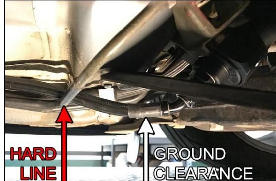
42. Using a 7/8" wrench, torque the 45 degree hose end on the fuel filter inlet first. Now torque the straight hose end on the pump hanger. To avoid breaking anything, brace the part. To prevent hose end marring, an aluminum wrench is recommended.
