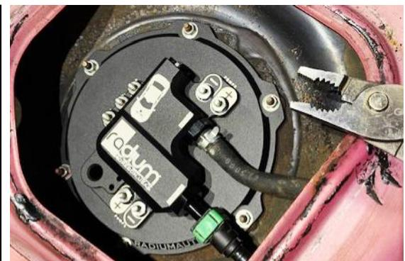
29. Send the OEM harnesses and pressure sensor from the interior back through the sheet metal hole and on top of the fuel tank. Reseat the rubber grommet.
