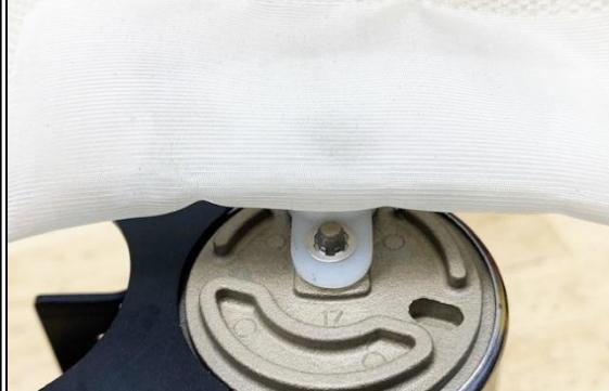
19. When dropping the assembled unit back into the collector box, the filter sock(s) might need to be folded for best clearance. Reinstall the collector box mounting screws.
