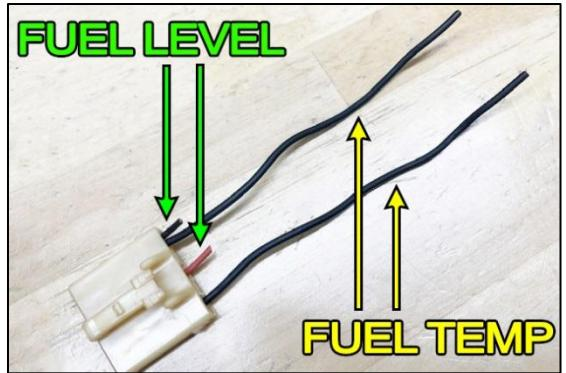
21. Strip all 4 wires from the fuel level sender and fuel temperature sensor. Next, crimp the 4 included terminals to each wire using a tool such as Molex 63811-1000 hand crimper. Slide the terminals into the plastic plugs until a "click" is felt. Polarity is not critical.
