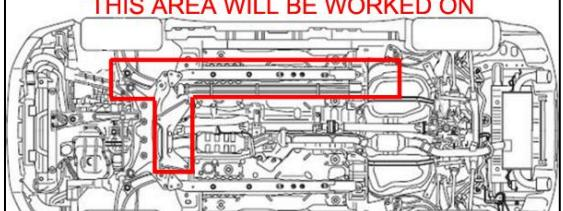
35. The plastic shield (pictured) near the left rear tire and the metal shield near the front left tire that covers the hard lines need to be removed temporarily. Using a 10mm socket wrench, remove the M6 screws and drop the shield down.
