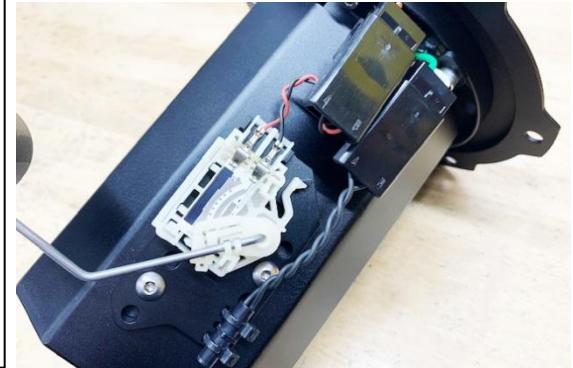
24. Using a 2.5mm Allen wrench, loosen the 2 button head screws (shown red) and remove the pressure sensor hold-down bracket (shown yellow).
