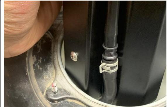
27. When dropping the fuel hanger down into the tank, be sure components such as the fuel level float, crossover hose (shown), sensor connectors, etc. do not get hung up.
