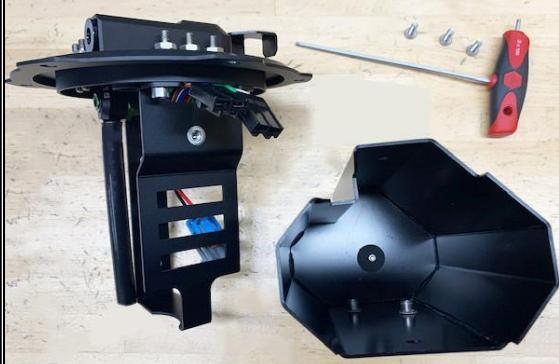
7. To remove the fuel pump bracket, unscrew the 3 socket head screws using a 4mm Allen wrench. NOTE: the fuel pump bracket may be a different color depending on the kit purchased.
