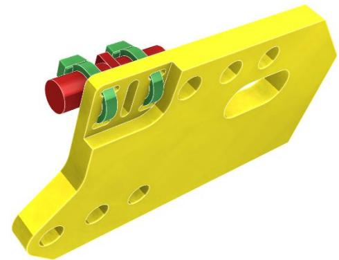
23. Reattach the Radium fuel sensor mount to the collector box. Next, carefully slide the OEM fuel level sensor downwards onto the mount until the tab locks into place.
