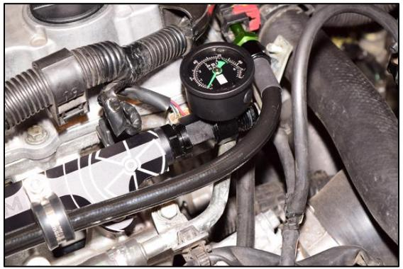
46. Reconnect battery. Turn key to ON position. Confirm new fuel pump(s) prime. If no leaks are found, start vehicle. The engine may run rough for a few seconds until all the air is bled from the fuel system. Recheck for leaks. Reinstall OEM metal cover (shown) and rear seat.
