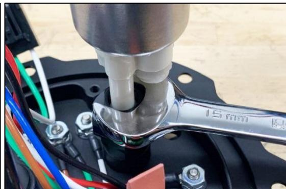
15. Reinstall the pump bracket. Allow the “fuel sensor” connectors to exit the pump bracket in the direction depicted (top of picture). This will setup for easier connections in a later step.
