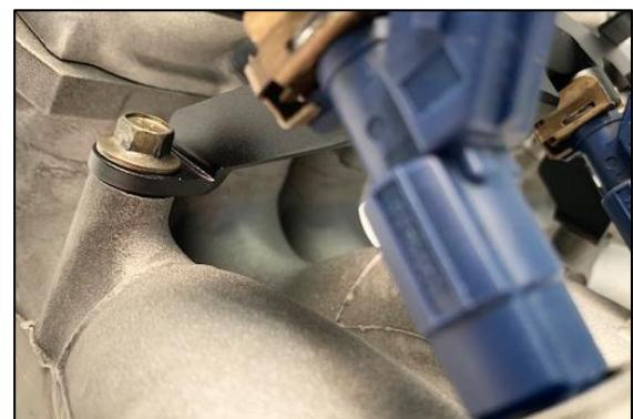
9. As a test, push the fuel injectors downward until they bottom out. Now inspect the injectors' upper O-rings and confirm they are still inserted into the fuel rail injector bores. Do not pressurize the fuel system until the proper height is achieved.
