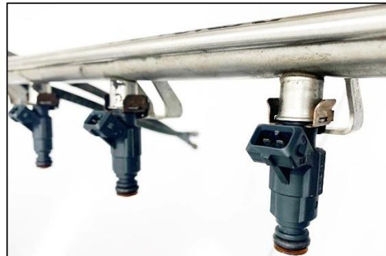
4. One by one, carefully unclip the fuel injectors from the OEM fuel rail. The OEM fuel injector locking clips will be reused.
