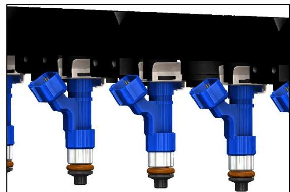
8. Lubricate the lower injector O-rings. Position the fuel rail assembly over the intake manifold. Press down until the injectors slide into the intake manifold ports.
