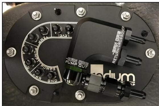
11. Be sure to use light oil lubrication for the O-rings prior to installing the fittings. Show is the correct fittings for the newer model Subarus.
