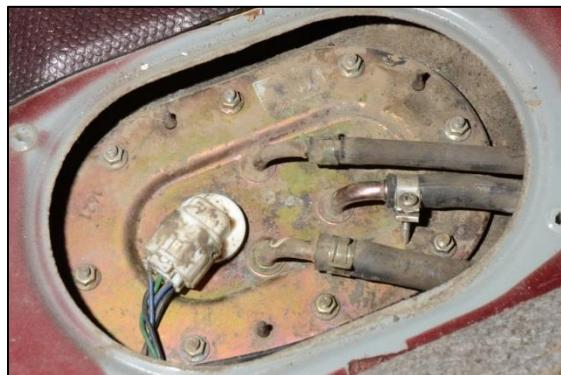
**3.** To reduce spills and make installation easier and safer, the gas tank should be drained.
