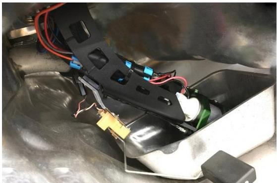
**25. Connect all 3 fuel lines (fuel feed, return, crossover). Light oil is recommended to be used on all of these connections. For older models, the OEM feed and return lines will need to be crossed to make the connections. For model years that use an SAE quick disconnect fuel feed, gently pull the OEM line to free up the necessary slack to make the connection. Be sure the SAE lock fully engages, as shown.**
