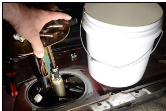
6a. Pull the OEM fuel pump housing out and drain into the bucket, as shown.
