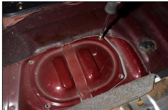
**2.** Once removed, it is recommended to clean the top of the fuel pump housing and the surrounding area. This will prevent loose dirt from falling into the gas tank.
