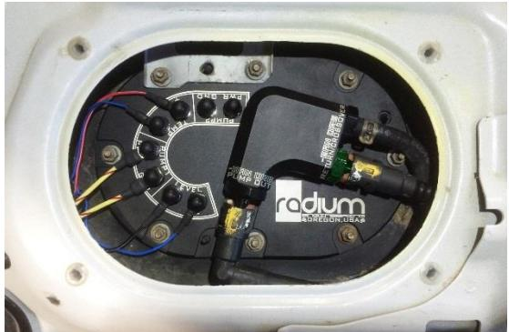
28. As shown, there are many wire color variations for all of the model years. Referencing the pinout chart, insert the ring terminals onto the corresponding studs.
