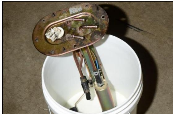
6b. NOTE: Subaru changed from external post-pump filters to internal post-pump filters around 2005 (depending on the model). This filter is easily identified as it is mounted directly to the fuel pump outlet, as shown.
