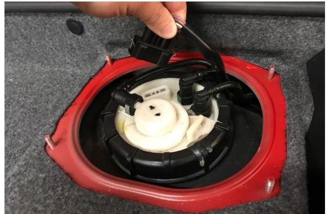
2. Temporarily install the large Radium mounting bracket attaching it to the 4 fuel pump access studs.
