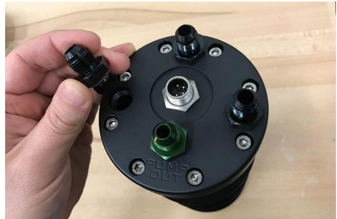
4. Remove the eight M5 bolts on the top plate of the fuel surge tank (FST) using a 4mm Allen hex wrench.
