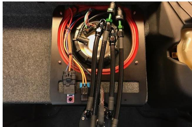
19. Reconnect the battery and turn the key to the ON position. Confirm that both pumps prime for a few seconds. Cycle the ignition several times to fill the surge tank. Check for leaks at all connections and correct any that may have occurred.
