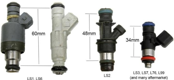
If using LS3/LS7 or aftermarket fuel injectors that are 34mm tall, you must install spacers on the injectors to increase the height from 34mm to 48mm. These spacers (or hats) are commonly available from most injector manufacturers and other performance parts retailers. See photo below as an example of a 34mm height injector with a spacer to make it a 48mm injector.
