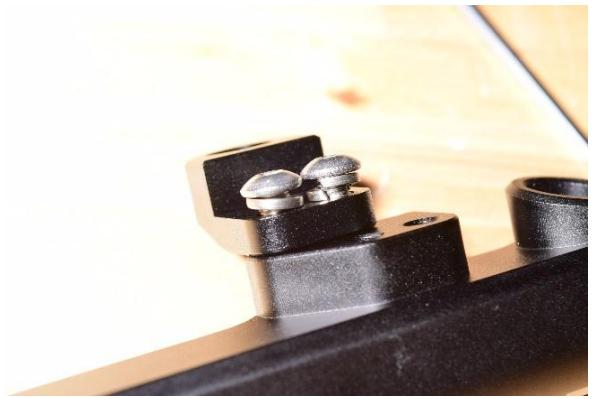
4. Install any fittings, plugs or accessories into the fuel rail ports. Lubricate all ORB O-rings with some oil to avoid damaging them.
