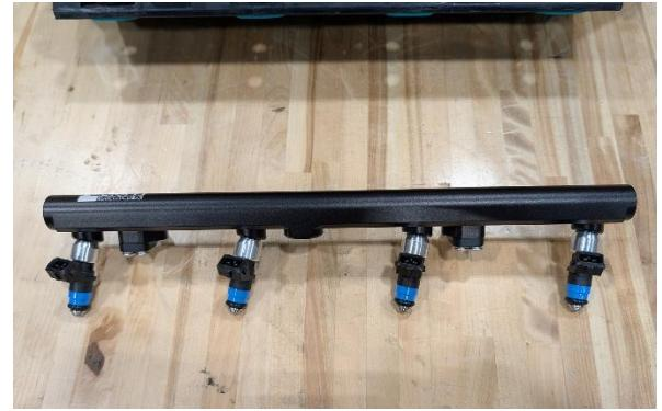
5. Clean out any dirt or debris found in the intake manifold injector seat bores and seat the fuel rails to the intake manifold.
