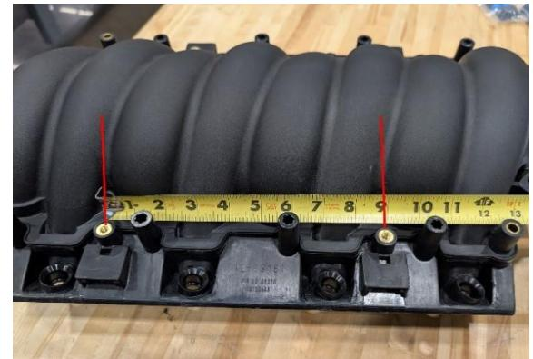
2A. If the spacing is closer to 8-1/4" (209mm), install the fuel rail feet on the inner holes, as shown.
