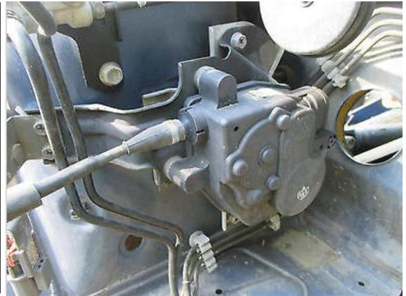
2. From the backside of the cruise control module, remove the 3 plastic-tapping screws holding the module to the OEM bracket.
