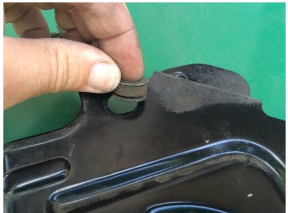
4. Install the rubber grommets into the Radium bracket. Mount the cruise control module using the OEM plastic-tapping screws.
