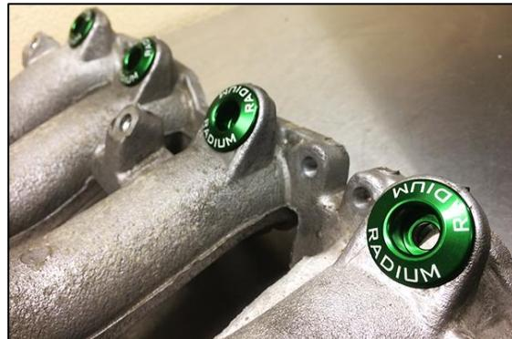
4. Radium Engineering injector seats for Subaru (22mm).
