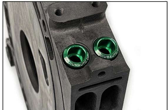
9. Radium Engineering injector seats shown for Mazda secondary rails.
