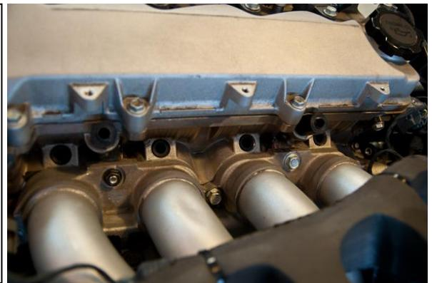
11. NOTE: If installing on a 2-Eleven or supercharged Exige-S with intercooler, some grinding is required of the intake manifold's aluminum boss as circled in the picture. **WARNING: DO NOT GRIND DOWN THE FUEL RAIL!**
