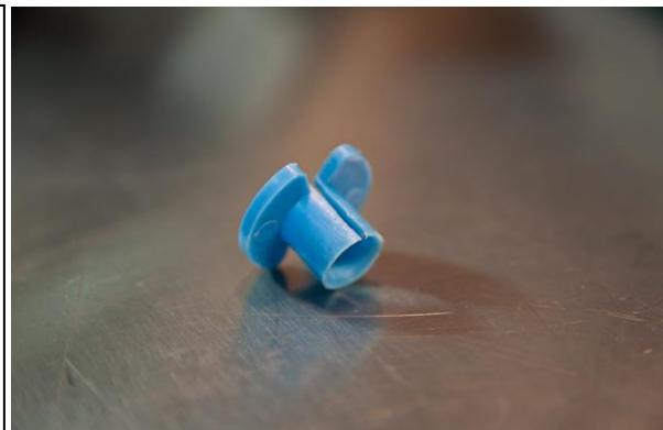
3. Insert the tool into the end of the fuel fitting. Make sure to surround the area with shop towels to absorb fuel contained in the pipe. While squeezing and applying pressure, pull the fitting away from the fuel pipe to release it from the fuel hose.
